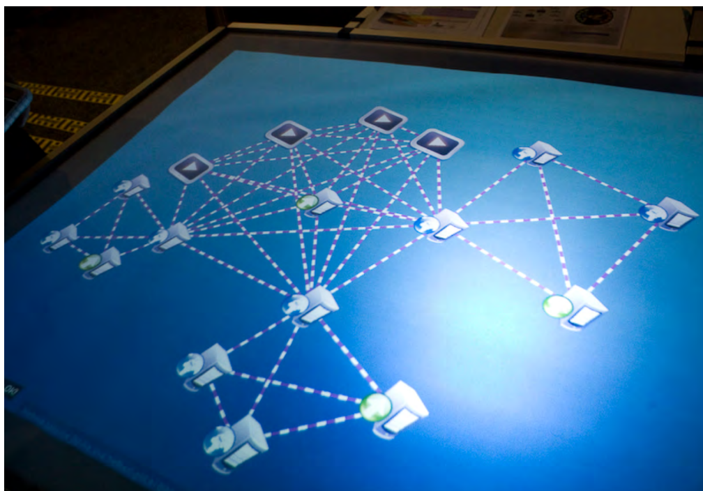
Figure 2. Network visualization after discovery. The dashed lines, when monitoring is enabled will indicate bandwidth (line width), delay (percentage of dashing) and jitter (randomize in dashing).
