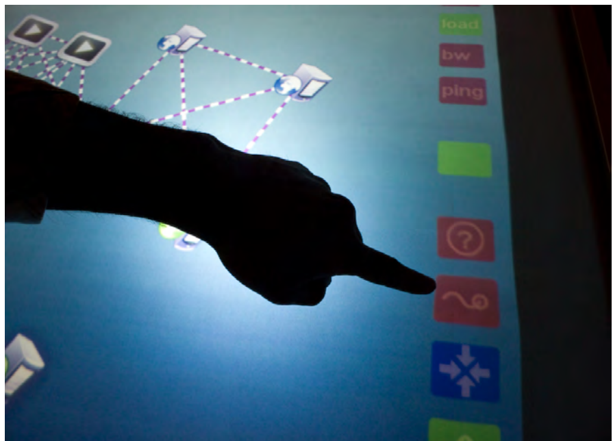
Figure 7. Changing path creation mode. The button with the question mark shows the discovered topology including non-programmable nodes.
