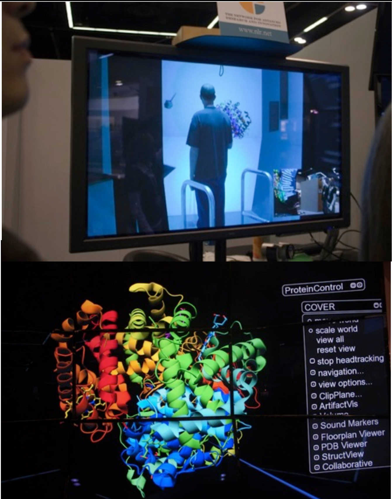
These photos from The KAUST Exhibit at Supercomputing 09 indicate the use of 3d visualization tools where two scientists can explore protein folding. In this instance they walk toward the display with a visor and a pointer that enables them to steer the display. They can communicate in real time examining the same model from different perspectives. The second picture shows a virtual navigation menu by means of which the user on the show floor can change his interaction with the display which uses eleven "tiled" LCD monitors, nine of which are visible.
